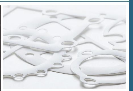
Durlon<sup>®</sup> Virgin PTFE gasket material is a high performance PTFE product designed for use in piping and equipment in chemical and other general industrial applications where resistance to highly aggressive chemicals (including hydrofluoric acid) is required. Virgin PTFE sheet material is available in two grades: Skived; has better physical properties, is a good electrical insulator, and FDA approved, and Reprocessed; recycled PTFE processed into skived or molded sheet.
